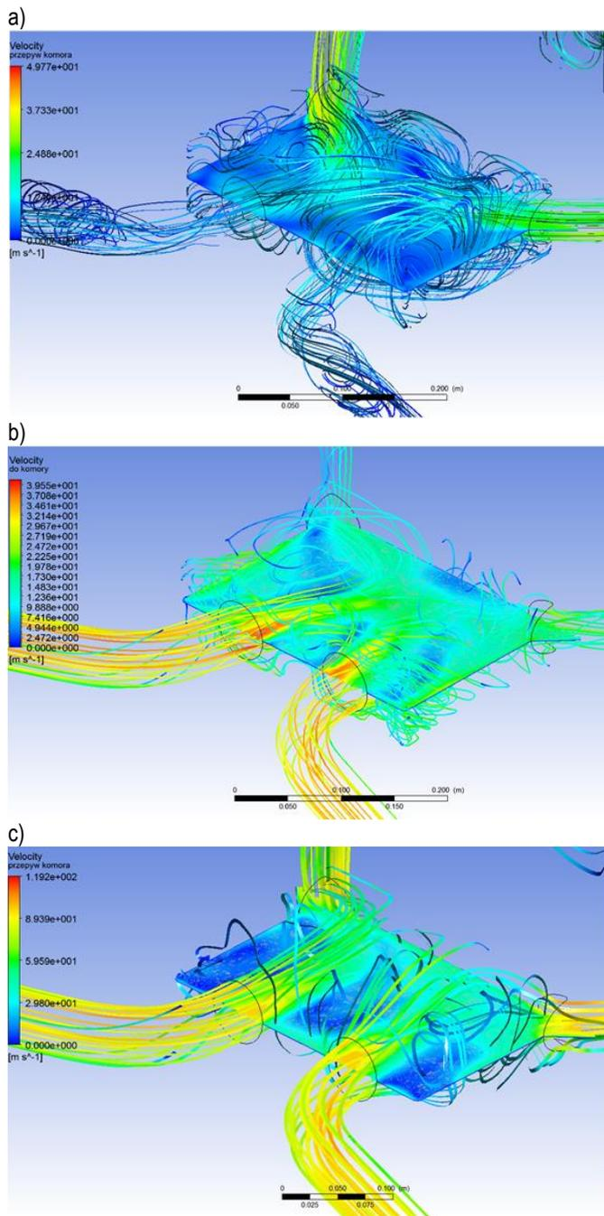
**Fig. 6.** Current lines between the inflow and outflow of medium in the filter chamber a)  $v_p = 0$  m/s; b)  $v_p = 36$  m/s; c)  $v_p = 94$  m/s
