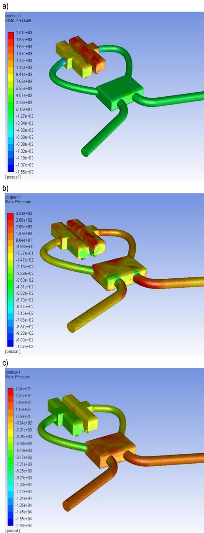
Fig. 4. Static pressure distribution a)  $v_p=0$  m/s; b)  $v_p= 36$  m/s; c)  $v_p= 94$  m/s
