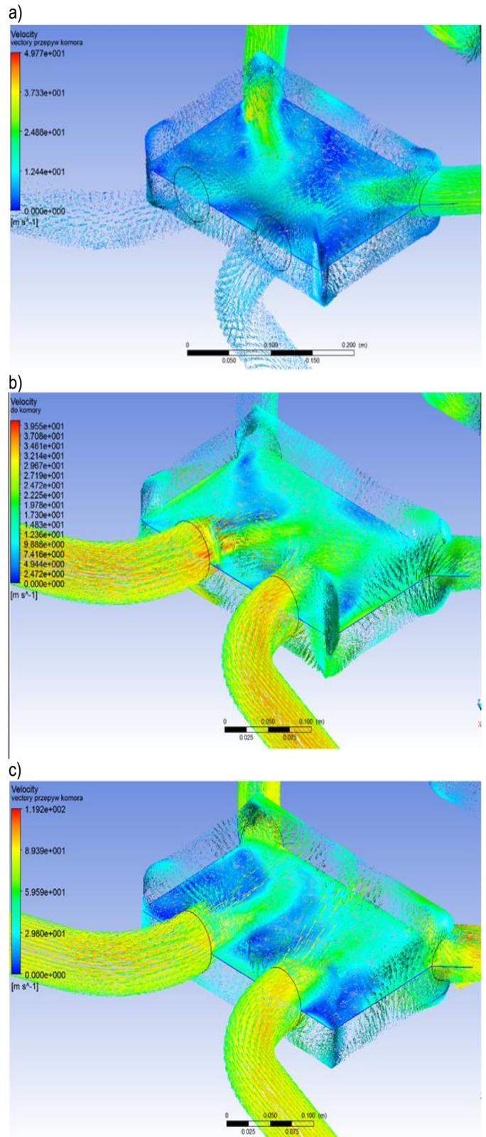
Fig. 5. Presentation of velocity and directions and returns of velocity medium in the filter chamber a)  $v_p=0$  m/s; b)  $v_p= 36$  m/s; c)  $v_p= 94$  m/s
