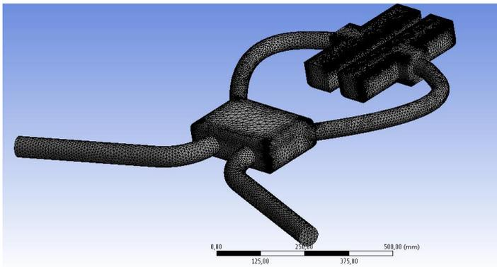
Fig. 2. Discrete model of the intake system of a Ferrari 348 GTC
