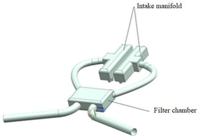
Fig. 1. View of the model of the intake system of the Ferrari 348 GTC sports car
