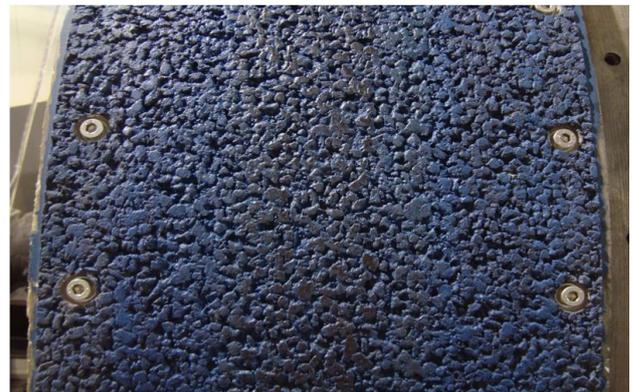
Fig.8. SMA8 surface replica (own material)
